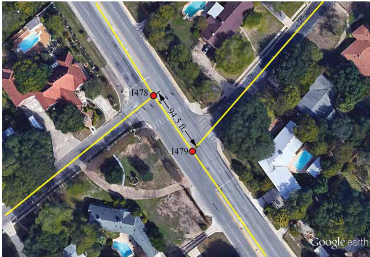
Figure 25. Intersection Offset Distance Measurement.
